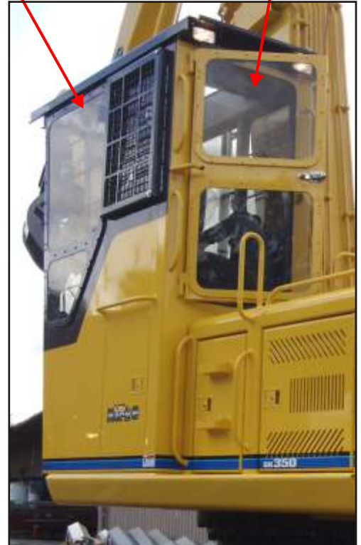
OPERATOR ESCAPE HATCH IN ROOF
